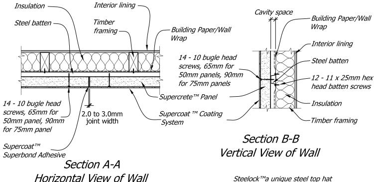
Steelock™a unique steel top hat batten mounting system. Thermoseal™ a unique thermally efficient closed cavity cladding system.
